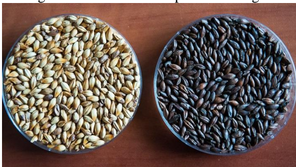
Figure 4. Malt before and after roasted in roasting drum with the developed new design.
