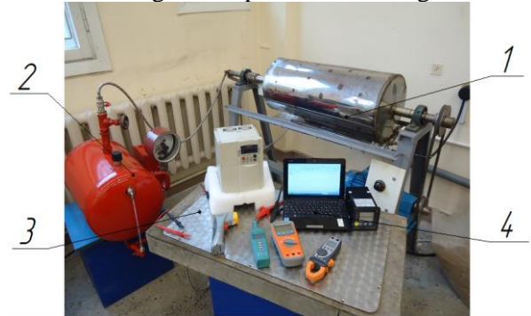
Figure 2. General view of the experimental stand 1 – fryer, 2 – steam generator, 3 – control equipment 4 – personal laptop ASUS 1005 PX.
