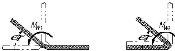
Figure 2. Moments of the resistance bending lines creasing cardboard boxing: a) unstrained bend line; b) pre- deformed line.
